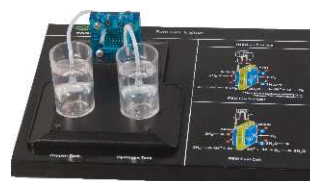
Reversible Fuel Cell and Gas Storage Tanks
