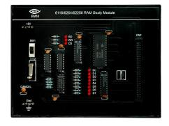
**EM01-EM10 Experimental Modules** are designed to study different peripherals used with 8085 and 8086 Microprocessors. This series is specifically targeting the 8085 and 8086 supporting peripherals. It covers Memory Elements, I/O peripherals and Timing and control devices of Microprocessor based system. With the help of these modules students can understand the interfacing and operation of peripherals. Ports are provided on Modules so students can use these ports to develop their own projects.
