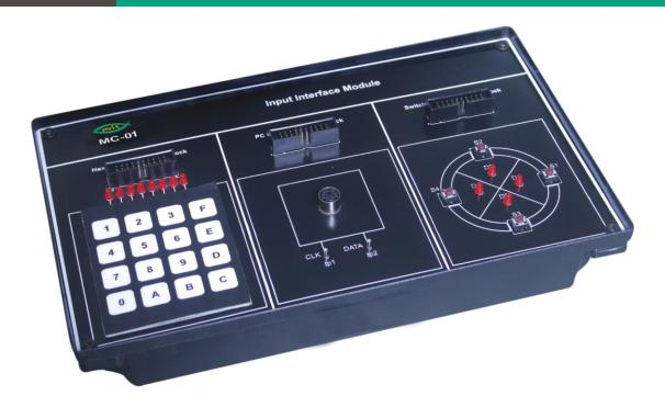
Input Interface module MC01 is an extension module for Nvis Microcontroller development platforms. The module has been designed for students and practicing engineers to gain invaluable practical experience on the principle and applications of microcontroller. The object is to have a clear understanding of how input peripherals are interfaced and controlled with microcontroller.
