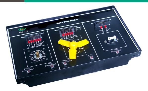
Motor Drive module MC05 is an extension module for Nvis Microcontroller development Platforms. MC05 has been designed to provide a clear understanding of how motors are interfaced and controlled with Microcontroller. The Motor Drive module is made in such a way that student can understand the detailed concepts of Stepper Motor, DC Motor, and Servo Motor system.
