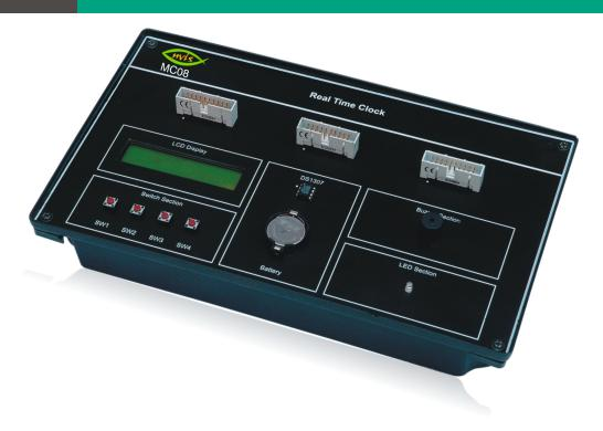
Real Time Clock module MC08 is an extension module for Nvis Microcontroller development platforms. It helps the user to gain invaluable practical experience of the principles and application of real time clock, LCD, switch and buzzer module in microcontroller based projects.
