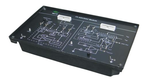
I<sup>2</sup>C protocol based ADC/DAC module enables students and practicing engineers to gain practical experience of applications of Microcontroller. The object is to understand how two wire serial interface device is used for interfacing with Microcontroller to communicate with external applications. Analog inputs are converted into digital through Microcontrollers and vice versa. ADC/DAC module, has input and output terminals for connection of external real world applications.
