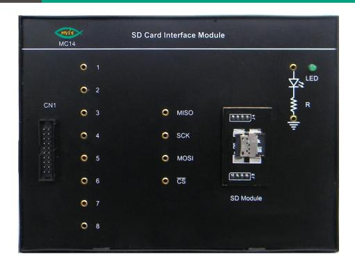
Nvis Technologies SD card interface module, MC14 is an extension module for Nvis Microcontroller development platforms. The object is to have a clear understanding of how Industry Standard SPI communication based SD card can interface and controlled with Microcontroller.
