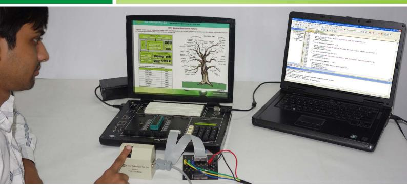
**Finger Print Module MC20FP** is an extension module for Nvis Microcontroller development platforms. The module has been designed for students and practicing engineers to gain invaluable practical experience on the principle and applications of microcontroller & Finger print module. The object is to have a clear understanding of how Finger print module is interfaced and controlled with microcontroller.
