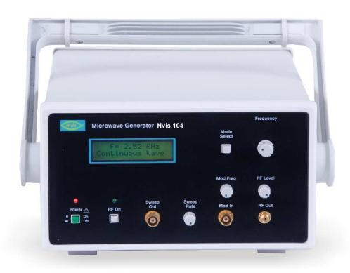
**Nvis 104 Microwave Generator** is a generator of frequency range 2.2GHz to 3GHz. It is a low cost and quality solution for microwave laboratories. It can be used as a source of 2.2GHz to 3GHz continuously variable frequency signal with Sweep, Internal AM, FM and External modulation modes. It is also used to study the characteristics of Micro Strip Component Designed in between 2.2 to 3GHz Microwave frequency ranges.
