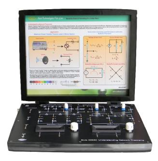
Nvis 6509C Understanding Network Theorems is a compact, ready to use experiment board and has been designed specifically for the study and verification of network theorems in DC circuits. In network analysis, the fundamental rules are ohm's law and Kirchhoff's laws. These laws may be applied to analyze any circuit configuration but for solving complex circuits, use of "Network theorems" is much better because it simplifies the analysis of complicated circuits.
