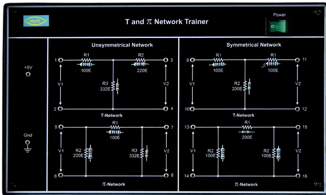
**Nvis 6518 T and  $\pi$  Network Trainer** has been exclusively and attractively designed to demonstrate the significance of image and characteristic impedance of T and  $\pi$ -network. It can be used as a stand alone unit with inbuilt DC power supply. Various scope of learning makes the subject understanding complete.
