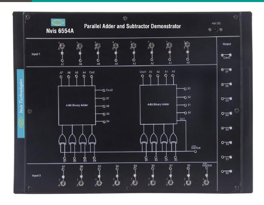
**Nvis 6554A Parallel Adder and Subtractor Demonstrator** is a ready to use digital electronics experiment trainer. This product has been designed specifically for the students to understand the concept of parallel binary addition and subtraction methods for 4 bit and 8 bit binary numbers.
