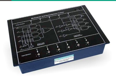
**Nvis 6556 Multiplexer and Demultiplexer Trainer** has been designed specifically for the study of 4-to-1 Line Multiplexer and 1-to-4 Line Demultiplexer. This Training Board familiarizes the students with the operation of both multiplexer and demultiplexer circuit. It explains the phenomena of Multiplexing of four input signals with two selection lines and one output. It explains Demultiplexing of one input signal with two selection lines and four outputs.
