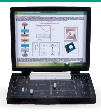
**Nvis 6577 PPM Modulation and Demodulation Trainer** is a very prominent training product designed for students to elucidate them the concept of Modulation and Demodulation. PPM is a method of encoding information in a signal by varying the position of pulses. The unmodulated signal consists of a continuous train of pulses of constant frequency, duration and amplitude. During modulation the pulse positions are changed to reflect the information being encoded
