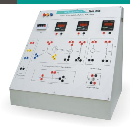
**Nvis 7036 Ward Leonard Method of DC Machine** is an elite training system for Electrical Laboratories. The product helps you to get fully acquainted with the basic concepts and functioning of a DC machines.
