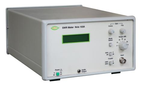
**SWR Meter Nvis 103A** is a Microcontroller based Equipment with LCD. The Analog metres have multiple scales which makes the instrument very complicated for the students. The Digital Display of SWR & dB solves the problem. Since the Equipment has a Microcontroller based digital display so there is no need of expanded scales, as it was in conventional instruments.
