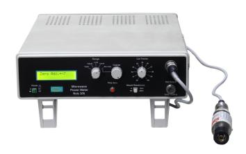
Nvis 105 Microwave Power Meter is an automatic self balancing power meter. It measures the RF power with the help of temperature compensated Thermistor Mount from 1µW to 10mW accurately. This provides the high accuracy over a wide temperature range by measuring the output voltage of the thermistor bridge and computing the corresponding power. The cable for connecting the sensor with the power meter is also provided.
