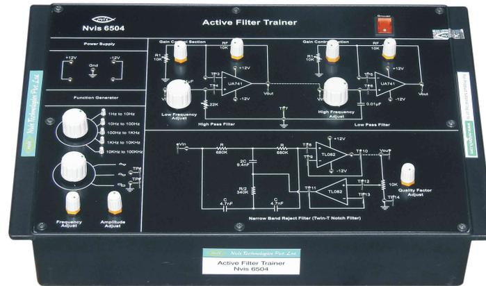
**Nvis 6504 Experimentation with Active Filters** is a remarkable and frequently used laboratory equipment which is designed to explain basic fundamentals of filter design and their working. Electronic filters are electronic circuits which perform signal processing functions, specifically intended to remove unwanted signal components and/or enhance wanted ones.
