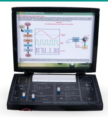
**Nvis 6576 PWM Modulation and Demodulation Trainer** is a useful training product for students to understand the concepts of Modulation and Demodulation. Pulse width modulation (PWM) is a technique used for controlling analog circuits with processor's digital outputs.
