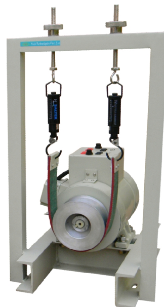
DC Motors with standard Mechanical loading arrangement
