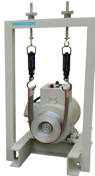
DC Motors with standard Mechanical loading arrangement
