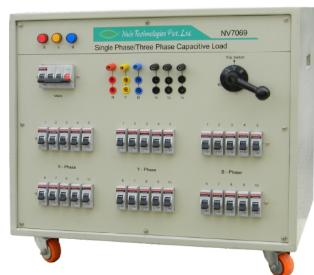
Single and Three Phase Capacitive Load
