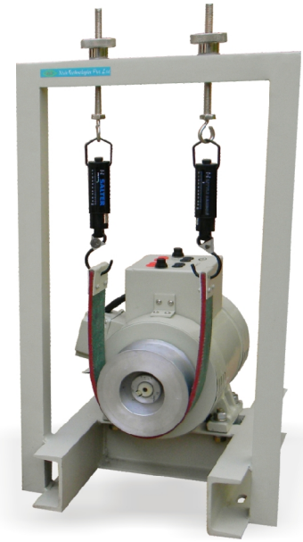
DC Motors with standard Mechanical loading arrangement
