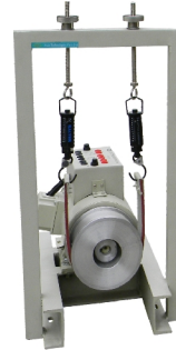
AC Motors with standard Mechanical loading arrangement
