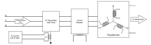
For understanding the role of relays in real time transmission system a circuit of transmission line is provided from source to distribution with proper placing of all its required components.
