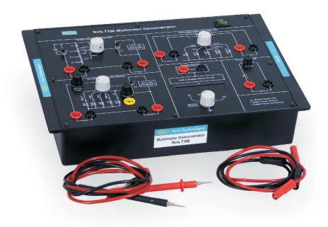
**Nvis 7106 Multimeter Demonstrator** is a versatile training product used in the electronic laboratories. With this Demonstrator students can easily understand the concept behind the measurement of different electrical quantities like Voltage, Current and Resistance.
