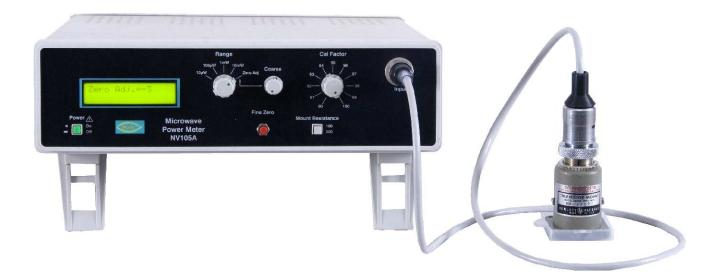
Nvis 105A Microwave Power Meter is an automatic self balancing power meter. It measures the RF power with the help of temperature compensated Thermistor Mount from  $1\mu W$  to 10mW accurately. This provides the high accuracy over a wide temperature range by measuring the output voltage of the thermistor bridge and computing the corresponding power. The cable for connecting the sensor with the power meter is also provided.
