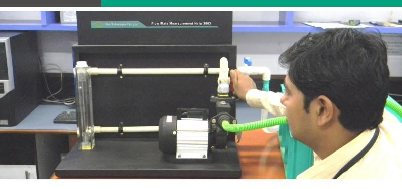
**Nvis 3003 Flow measurement** using a Rotameter exposes student and industry professionals to fundamentals of flow rate measurement. Its demonstrates how a Rotameter can measure flow rate of water.
