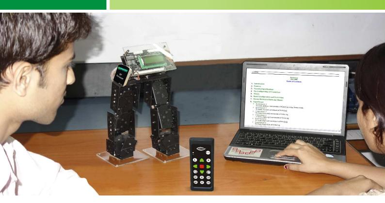
**Nvis 3305 RoboLeg** is a next generation legged robot platform with marvelous design and capabilities. It has 6 degrees of freedom which gives it stable walking steps using 6 servo motors. The main board of the RoboLeg can drive up to 6 servo motors in parallel. There are various ports, I2C, SPI and USART connectors for variety of applications like sensor interfacing.
