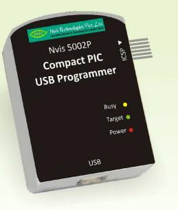
**Compact PIC USB Programmer Nvis 5002P** is designed for Microchip PIC10F/12F/16F/18F series microcontroller with full featured USB in-circuit serial programmer (ICSP). This USB Programmer will easily connect with PC & laptops. It comes with programmer software which allows user to perform various commands like Read, Erase, Write, Verify, Blank check.
