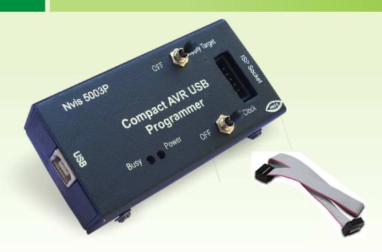
Compact AVR USB Programmer Nvis 5003P is designed for ATMEL ATmega, Tiny & AT90 series Microcontroller. It is a full featured USB in-circuit programmer for Atmel AVR microcontrollers. This USB programmer will easily connect with PC and laptops. It comes with Programmer Software which allows user to perform various commands like Read chip signature, Erase, Read/Write, Verify and Fuses/Lock bits setting.
