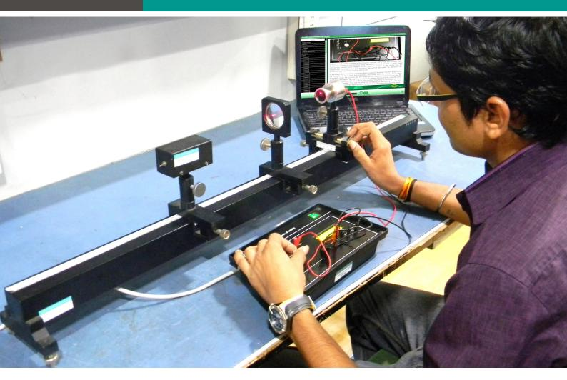
**Nvis 6006C Divergence of LASER** is an Optical setup helpful to identify characteristic of LASER beam. This product illustrates how the spreading of LASER beam enhances with respect to distance travelled in a medium. Nvis 6006C consists of Optics Bench and Measurement unit. The Measurement unit consists of variable DC power supply, voltage and current display. The Optics Bench consists of LASER source, Converging lens and Photo detector with distance measurement arrangement.
