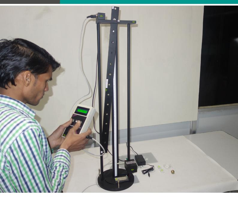
**Nvis 6051 Acceleration Measurement Setup** is very useful to understand the concept of Gravitational force of earth. It includes Simple Pendulum, Compound Pendulum and concept of object drop method.
