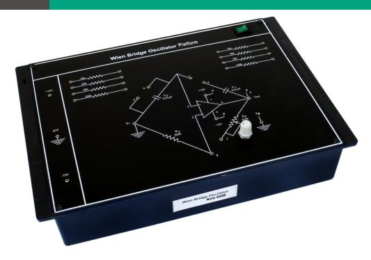
**Nvis 6506 Understanding Wien Bridge** is an elite training system for the analog electronics laboratories. It is useful in understanding the basic concepts and functioning of the oscillator and its use in generation of sinusoidal waveform.
