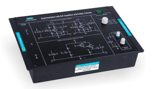
**Nvis 6542 BJT Experimentation with Amplifiers and Emitter follower** is a unique product designed to explain the role of BJTs as Single Stage/Multistage RC-coupled Amplifiers and as a Common Collector Emitter Followers.
