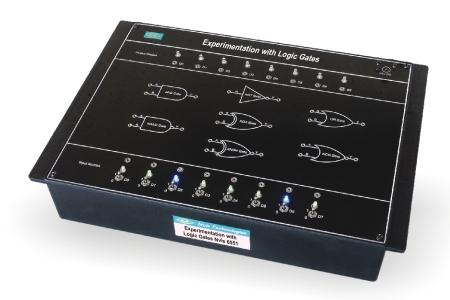
**Nvis 6551 Experimentation with Logic Gates** is an elite training system for the digital laboratories. It is useful in understanding the basic concepts and functioning of logic gates and their truth tables.
