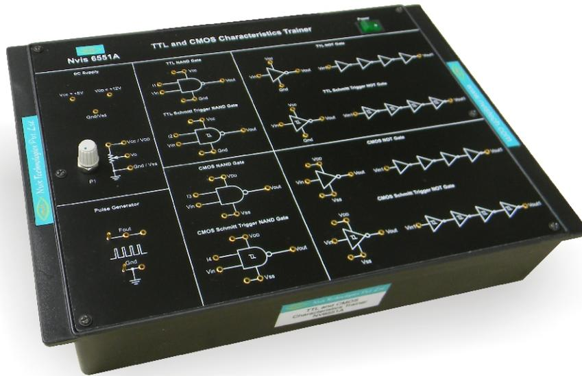
**Nvis 6551A Experimentation with Characteristics of TTL and CMOS** is a compact product designed to explain the fundamentals of Transistor–Transistor Logic (i.e. TTL) and Complementary Metal Oxide Semiconductor (i.e. CMOS), like Voltage Transfer Characteristics, Noise Margin and Gate Delay. Inbuilt Function Generator and DC supply is provided for ease of operation.
