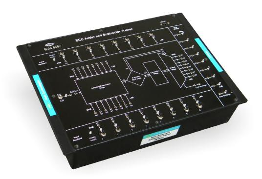
**Nvis 6562 BCD Adder and Subtractor Trainer** is a compact, ready to use digital electronics experiment board. This product has been designed specifically for the students to study and understand the concept of BCD addition and subtraction processes.
