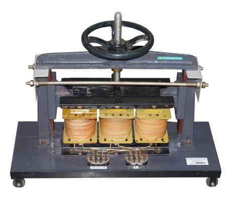
**Nvis 7068 Three Phase Inductive Load** is suitable for loading Three Phase supplies and generators. It consists three variable inductive coils. Two terminals for each phase are given which are externally accessible. A movable handle is used to change the inductance of the load.
