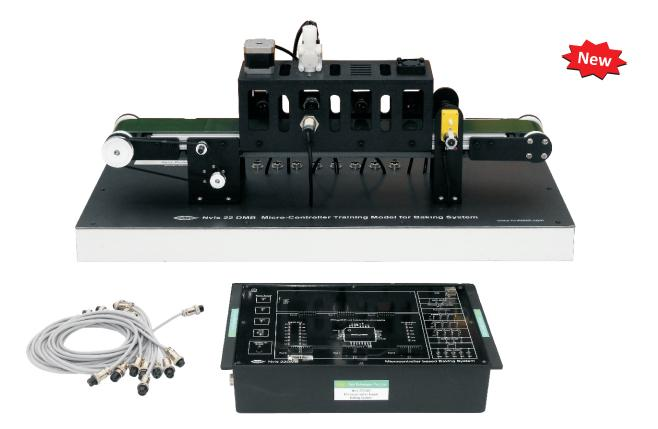
**Nvis 22DMB "Microcontroller based Baking System"** is designed to provide practical hands-on experience with microcontroller programming and interfacing. It is a popular tool used in educational institutions and industry for teaching and learning microcontroller concepts.
