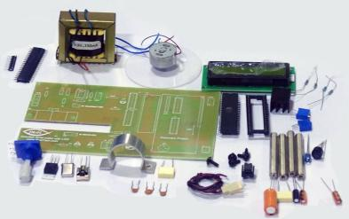
In this circuit microcontroller AT89C52 measures and shows on an LCD the RPM of a running motor. Counting the revolutions per minute (RPM) of motor i.e. determining the motor speed, is essential in the field of industrial automation. The number of revolutions per minute (rpm) is valuable information for understanding any rotational system.
