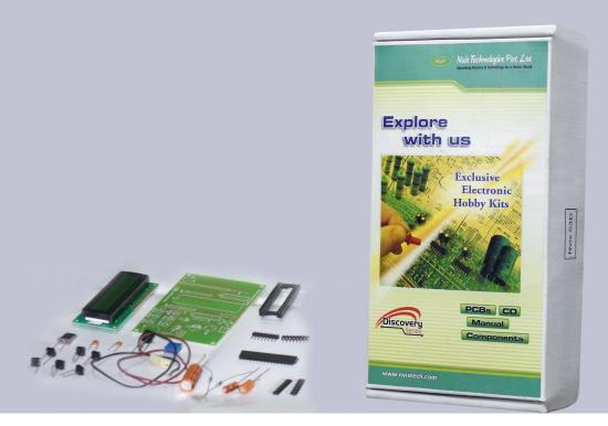
The Timer circuit consists of two parts one is Up Timer and another is Down Timer. User can set the time maximum up to 0 sec to 60 minutes (up timer) & 60 minutes to 0 sec (down timer). Buzzer is provided on the PCB, which will turn on when set time is completed.
