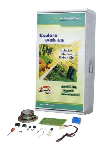
The Simple Musical bell uses IC 555 timer that operates in monostable mode. The circuit uses IC called UM66 which is a Musical IC and produces a melody sound at the output using speaker. As the switch is pressed the 555 timer gets activated and speaker produces sound for at least 15-20sec.
