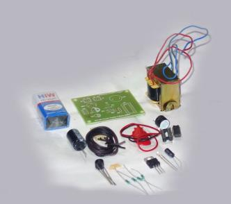
Power supply failure alarm circuit is useful in such application where we need continuously power supply. This circuit will generate an alarm and LED will glow when mains supply is turned OFF. The user came to know that mains supply is failed and the user can arrange alternate supply. This circuit is build using OP-AMP IC LM 324.
