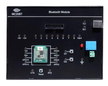
Bluetooth MC20BT Module is an extension module for Nvis Microcontroller development platforms. The module has been designed for students and practicing engineers to gain invaluable practical experience on the principle and applications of microcontroller & Bluetooth module. The objective is to have a clear understanding of how Bluetooth module is interfaced and controlled with microcontroller.
