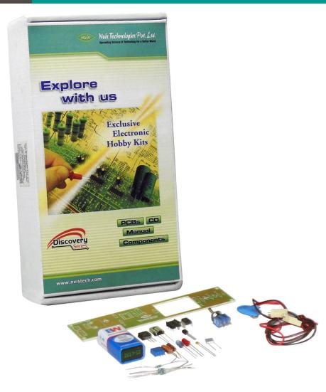
An infrared (IR) switch is a type of switch that allows users to turn another device on or off. An IR switch requires an IR signal to work. An IR switch is divided into two parts namely transmitter and receiver. The transmitter generates a 38 KHz frequency with the help of 555 timer and hence allows IR led to transmit IR rays at this frequency. The IR rays are received at receiver by ICTSOP 1738.
