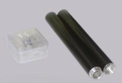
Eddy current kit facilitates an easy way to understand the concept of eddy current and Lenz's law. Here we produce the changing magnetic field through the freely falling magnet due to which eddy current is generated in the conductor which creates a magnetic field that opposes the falling of magnet
