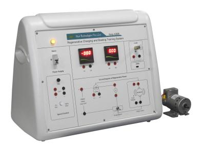
Energy saving and extended mileage are very important for battery-operated electric vehicles (BEV). Regenerative braking performances are the key for saving energy in BEV's. Nvis 438R training system introduces Permanent Magnet DC (PMDC) motor based regenerative braking to improve energy efficiency in BEV. The kinetic energy of the motor is returned to the battery system in regenerative charging.
