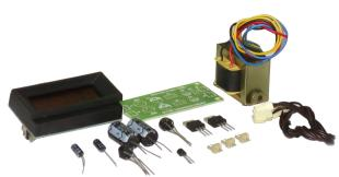
Temperature indicator is very easy to build. It shows temperature on digital panel meter (DPM). This circuit is build using temperature sensor LM 35 and DPM and few discrete component. Temperature sensor LM 35 generates the output 10mV/Centigrade. Temperature sensor generates output voltage which will be read by DPM.
